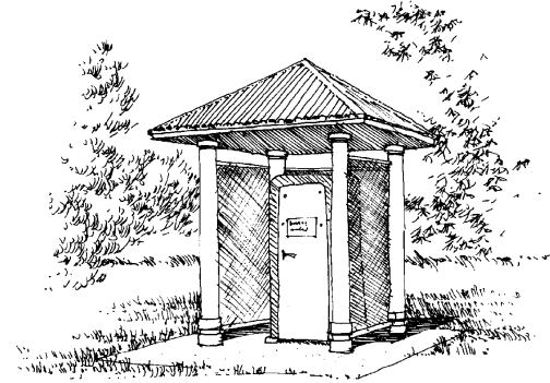
Chemical Toilet Concept (Sized to be Wheelchair Accessible)
